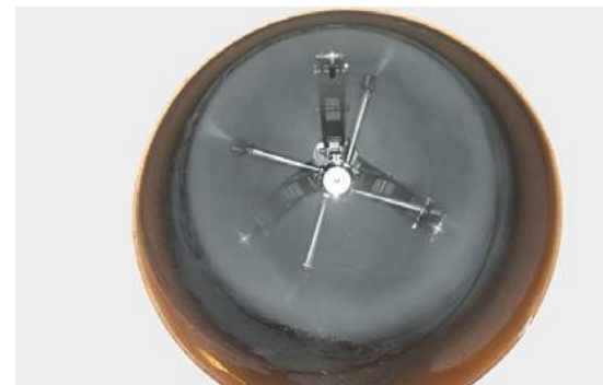
High pressure cleaning unit
