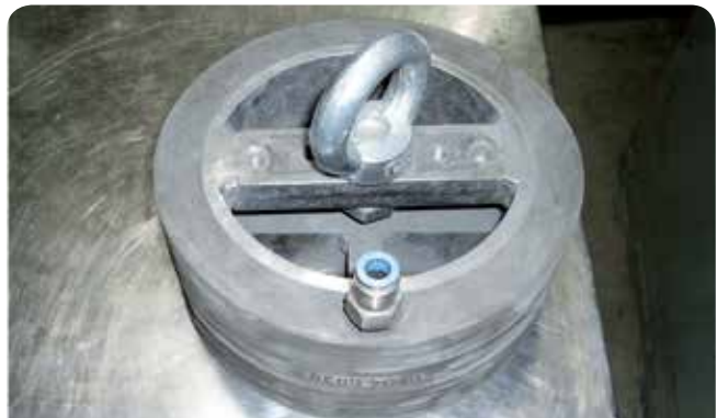
Pipe grip with external expansion
